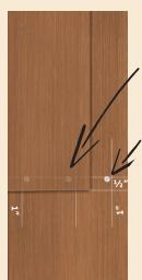
Use 2 fasteners for 4", 5", and 6" wide shingles
