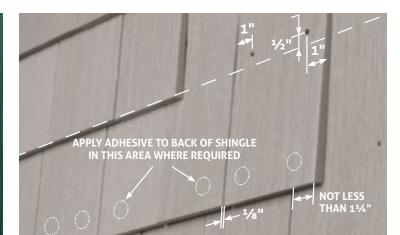
Use 2 fasteners for 4", 5", and 6" wide shingles (4" wide only available in 13" shingles)
