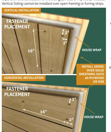
Along the length: **Fasteners** no farther apart than 16" 16" 16" Use additional fasteners in center as shown 16" 16" Exactly 2" from the end of the board 4" WIDE 8" WIDE 6" WIDE 10" WIDE
