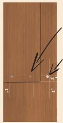
Use 2 fasteners for 4", 5", and 6" wide shingles (4" wide only available in 13" shingles)
